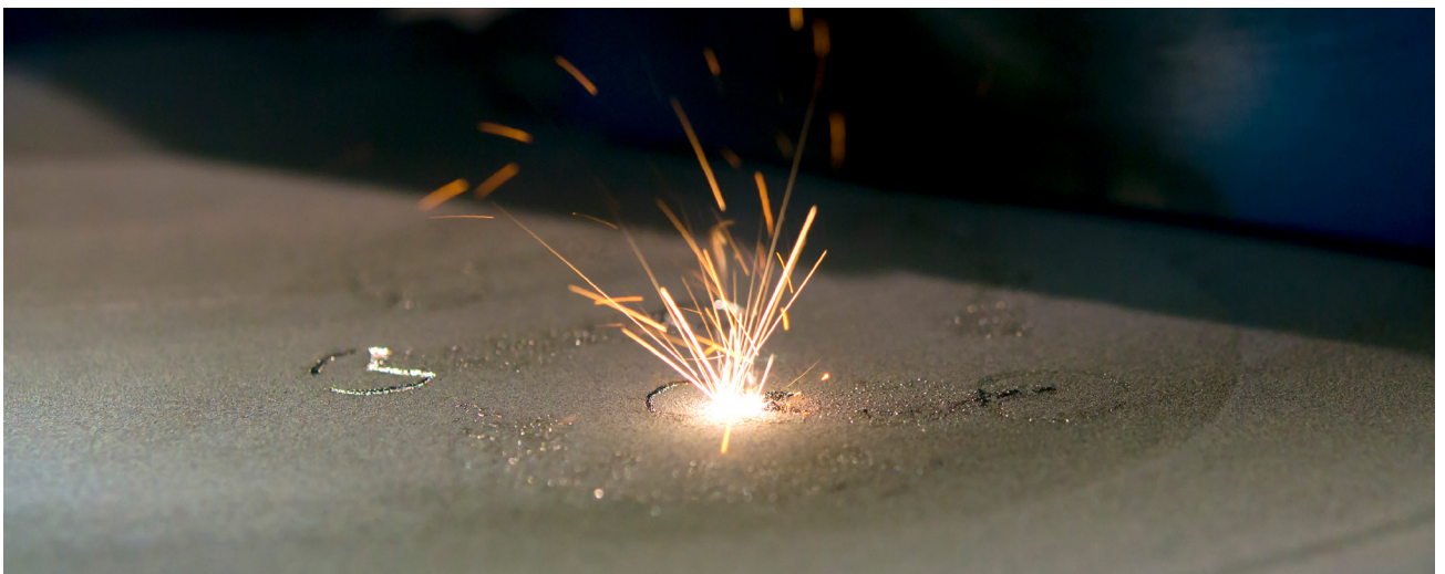
DMLS and SLM 3D printers use a powerful laser to build up layers of melted metal powder
