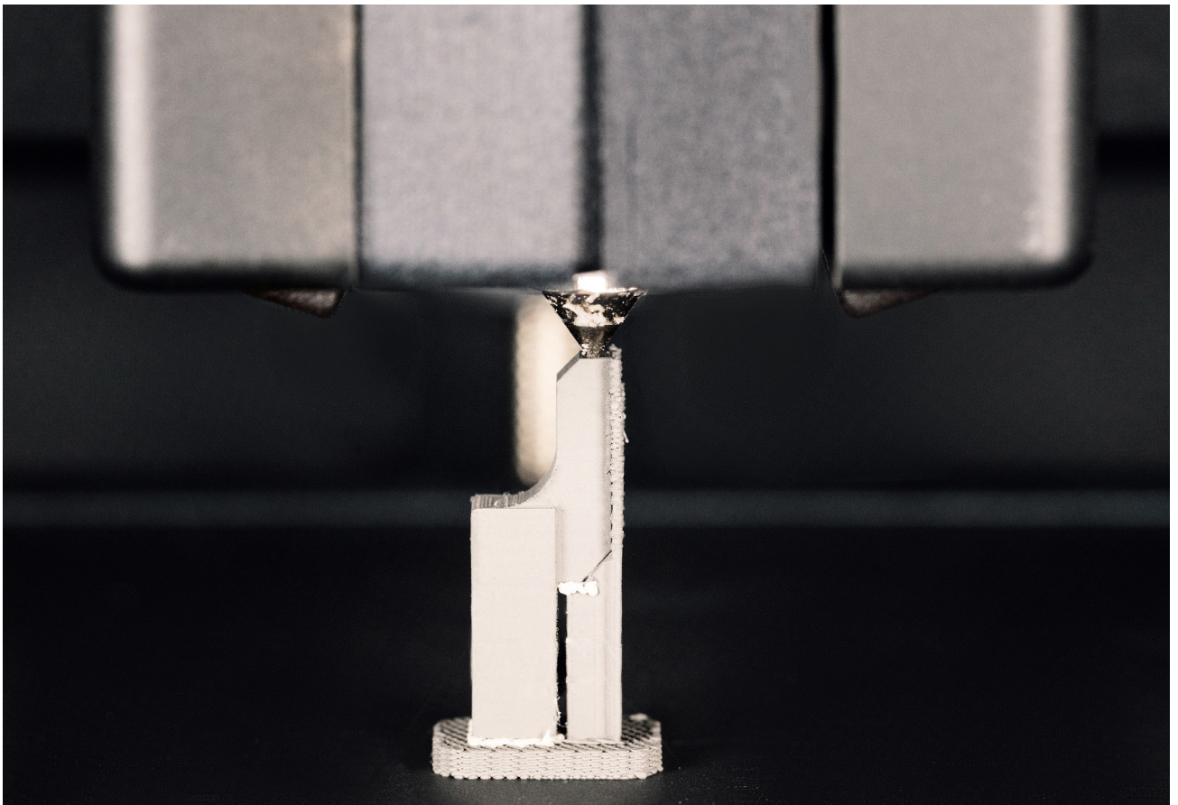
BMD printers extrude metal-polymer rods in layers to form a 'green part', which must be debound and sintered
