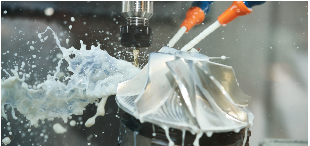
5-axis CNC machines are cheaper than metal 3D printers, but subtractive manufacturing limits geometric freedom
