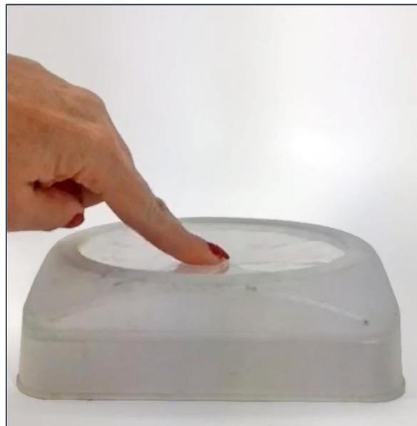
*In the image above, a touch from a finger can cause flexible build trays to move, showing how prone they are to distortion during an active 3D print build.*
