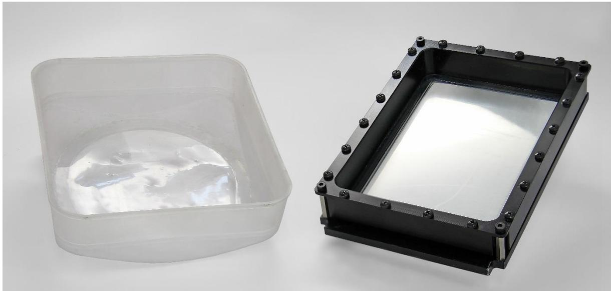
*The quality of the material tray used during 3D printing can have a significant impact on the quality and accuracy of the final part, because light must travel through the bottom of the tray to cure an even layer of resin across the build platform. On the left, a used material tray from a budget 3D printer. On the right, a robust material tray from EnvisionTEC that is made with optical glass and an aluminum frame.*
